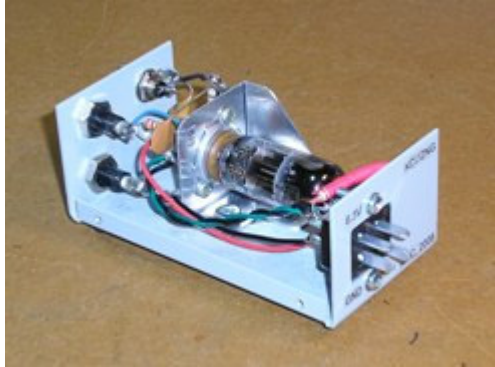
Figure 2. The inside of the unit, as seen from the back. A homebrew bracket holds the tube socket and a Jones connector accepts power from an external supply.
