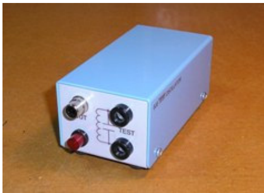
Figure 3. The completed test oscillator, from the front, with ink-jet decal labels.
